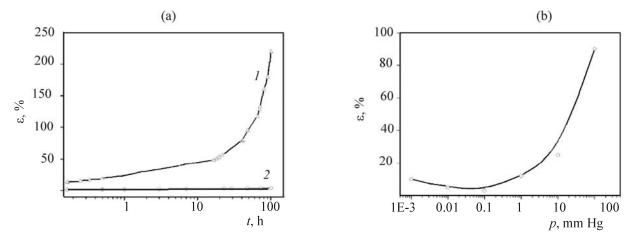
**Fig. 2.** Variation of strain (a) with time for (1) initial and (2) modified polytetrafluoroethylene film in the creep mode and (b) with oxygen pressure in the reaction chamber for modified film. Film thickness 100  $\mu$ m, test portion width and length 5 and 20 mm, respectively; load 11 MPa; working temperature 18–20°C. Modification conditions: absorbed dose 200 kGy; oxygen pressure  $10^{-1}$  mm Hg.
