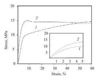
**Fig. 3.** Stress–strain curves for (1) initial and (2) radiationmodified polytetrafluoroethylene. Insert: stress–strain curves in the region of low strains. Absorbed dose 200 kGy; oxygen pressure in the reaction chamber  $10^{-1}$  mm Hg.
