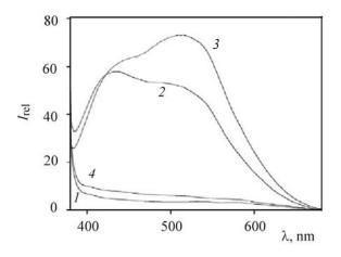
**Fig. 4.** Fluorescence spectra of modified polytetrafluoroethylene under excitation at  $\lambda = 365$  nm. Absorbed dose 200 kGy, and oxygen pressure, mm Hg: (1) 10<sup>-3</sup>, (2) 10<sup>-1</sup>, (3) 1, and (4) 100.
